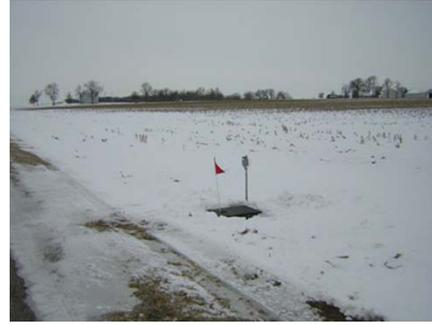
For *overland runoff*, a weir is installed to measure flow volume and allow for sample collection.
